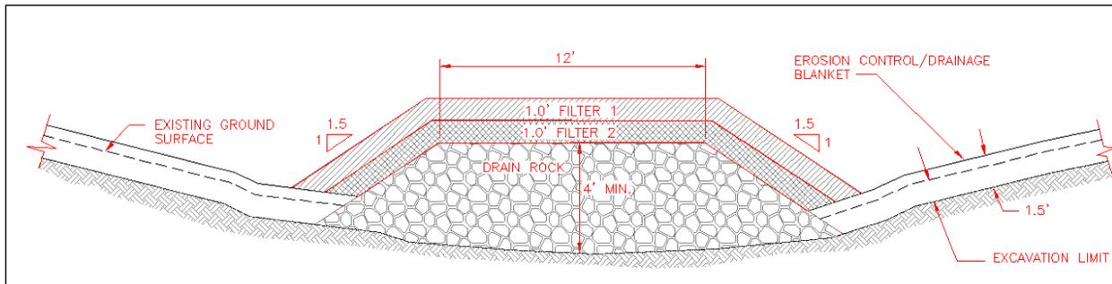
**Figure 2: Typical Cross Section of Flow-Through Drain**
